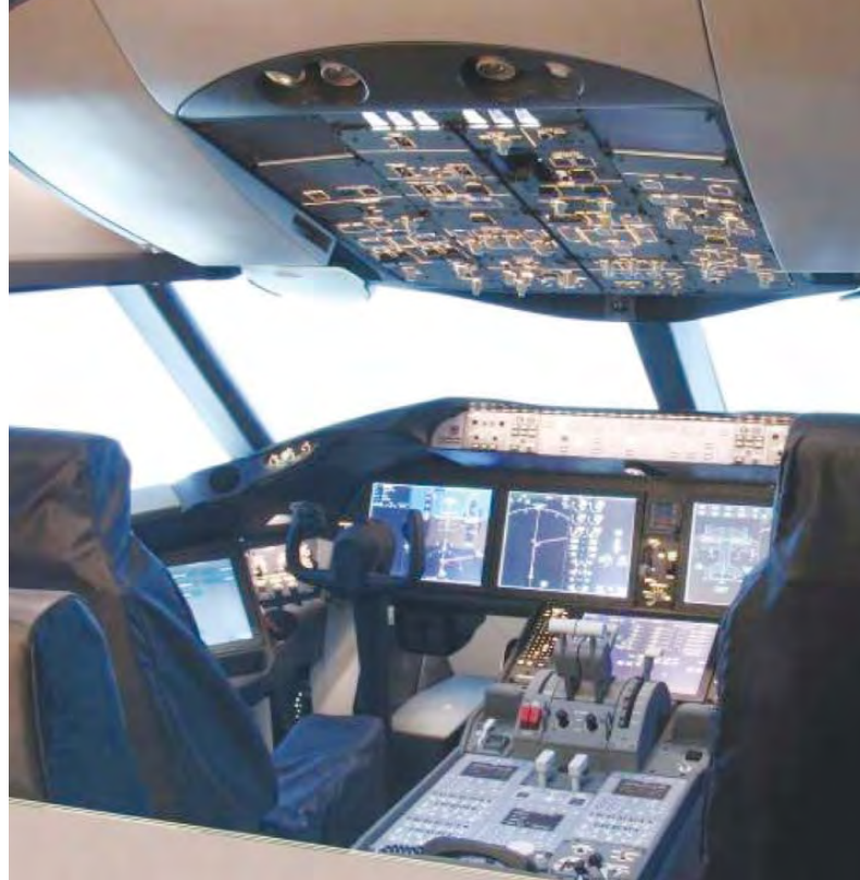
One of several flight deck mock-ups used in development - this one is a full-systems validation rig.
